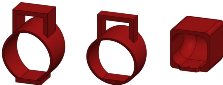
Figure 12: Design of the proximal, middle and distal index finger phalanges
