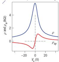
The longitudinal resistivity  $\rho$  reaches its maximum value at the Dirac point. Away from Dirac point the dependence on gate voltage can be considered as linear. The Hall resistivity  $\rho_{xy}$  has two maxima. The positive (negative) sign of the maximum indicates electron (hole) doping. In the vicinity of the Dirac point,  $\rho_{xy}$  has the steepest slope.
