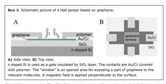
The Hall bar geometry (Box 3) of electrical contacts allows achieving the highest sensitivity towards adsorption of molecules. The design idea of the device consists of a "window" that opens a part of the graphene flake for exposure to molecules, and the system of electrical contacts isolated from each other and the molecules.
