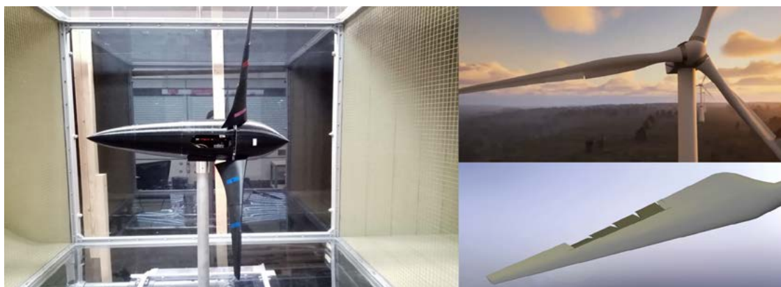
Experimental turbine with partially oscillating blades in the ESRIG windtunnel (left), Artist impression of modified Vestas V-52 turbine (right).
