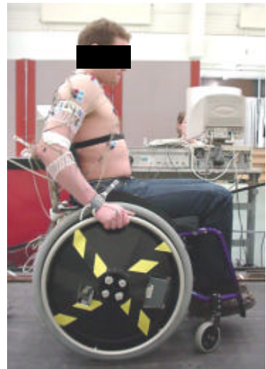
Figure 1.2: Subject in the instrumented wheelchair during level wheelchair propulsion at 3 \text{ km}\cdot\text{hr}^{-1} .
